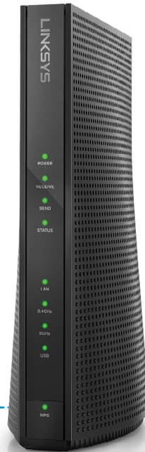
CABLE MODEM ROUTER Converts data to Ethernet / WiFi
