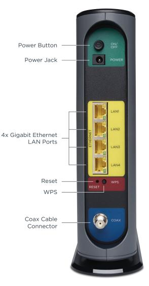
This cable modem/router does not have telephone jacks for support of voice phone calls.
