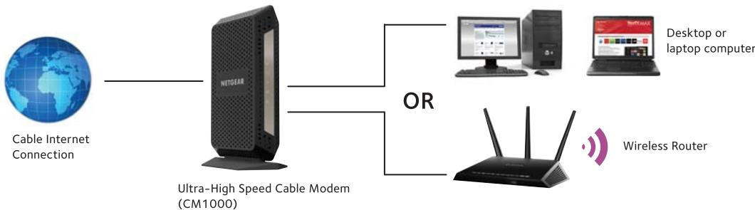
Connect the CM1000 Ultra-High Speed Cable Modem directly to your computer or wireless router for connecting to other wireless devices.
